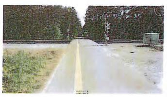
The Koppers Road Extension is currently a twenty-two foot (22) to forty (40) foot wide Florence County Asphalt and Dirt Roadway extending approximately 7,300 linear feet from US Highway 76 to Old Marion Highway. The existing asphalt section of Koppers Road Extension is approximately 2,100 linear feet
